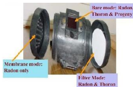
Figure 2. Radon-Thoron mixed field dosimeter system
