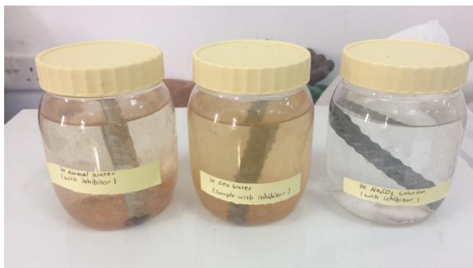
Figure 6: Samples dipped in the corrosive liquid medium
