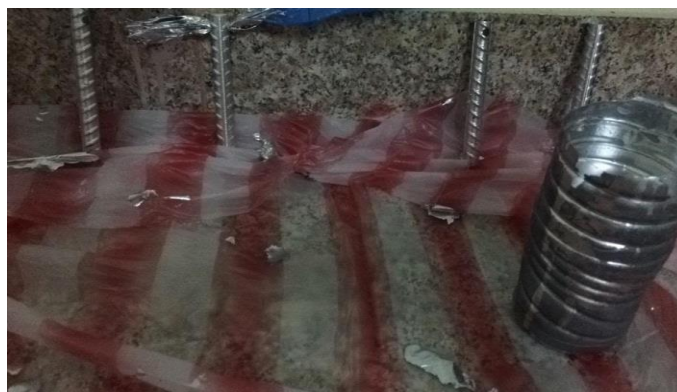
Figure 3: Mild steel coating with aluminum paint without inhibitor
