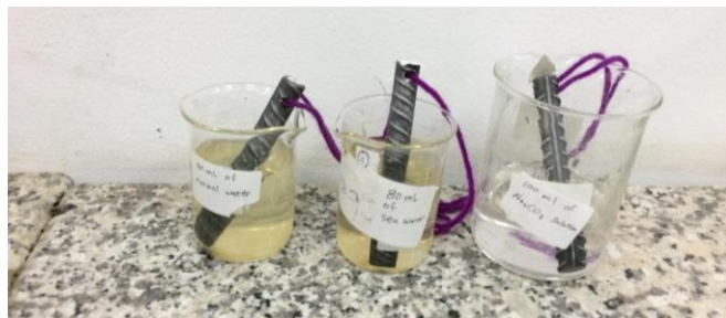
Figure 1: mild steel samples dipped in different in corrosive medium
