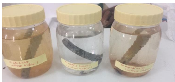
Figure 4: Samples dipped in different corrosive liquid medium
