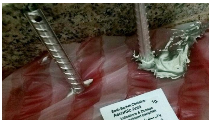
Figure 5: Mild steel coating with aluminum paint and inhibitor
