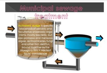
**Figure 4:** Sketch of secondary sewage treatment in activated sludge tank connected with secondary clarifier (activation – intensification of processes ongoing in nature)
