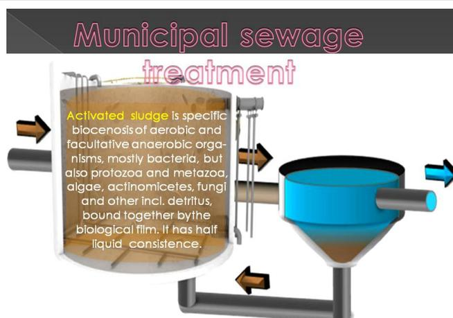
**Figure 4:** Sketch of secondary sewage treatment in activated sludge tank connected with secondary clarifier (activation – intensification of processes ongoing in nature)
