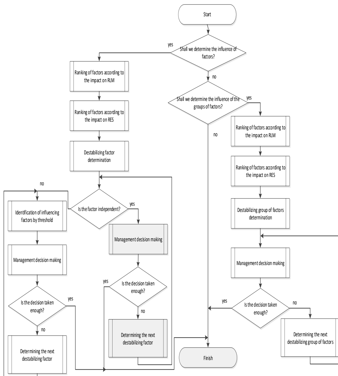
Figure 4: Algorithm of managing a single factor, an aggregate or a group of factors
