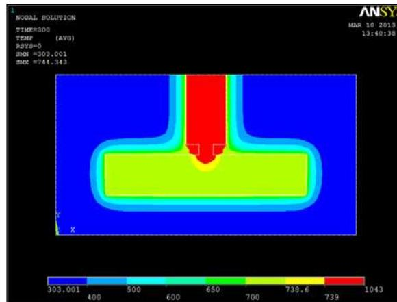
**Fig. 14. Location of Hot Spot for Riser with Diameter 40**
