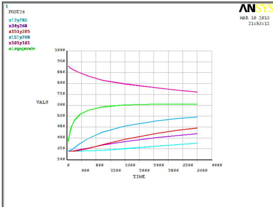
Fig. 19. Temperature Time Plot for Casting with Air Gap
