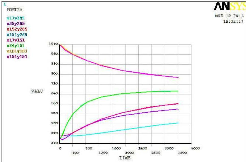
Fig. 11. Temperature Time Graph for PLANE 77 element
