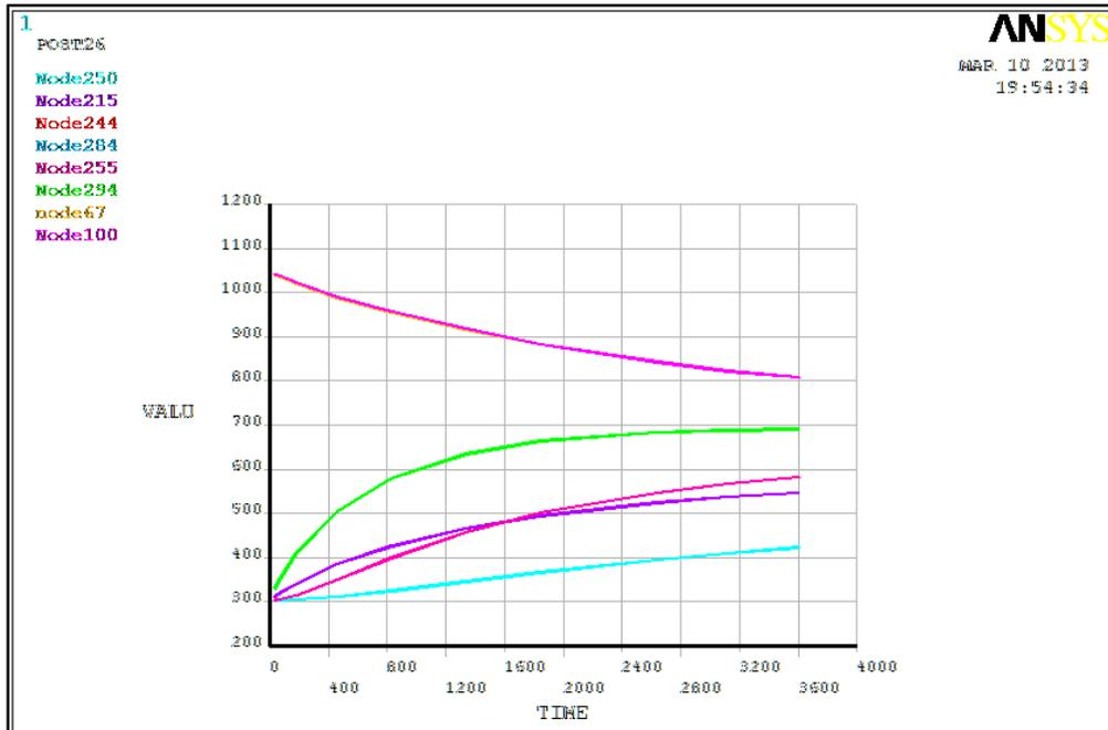
**Fig. 7. Temperature Time Plot for Free Mesh**
