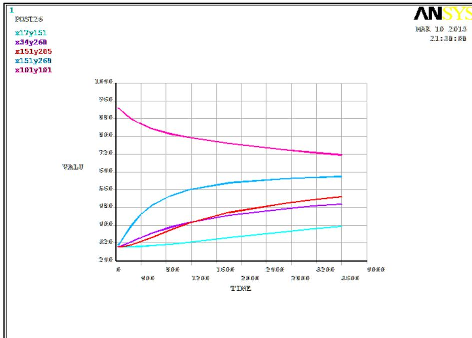
Fig. 20. Temperature Time Plot for Casting without Air Gap
