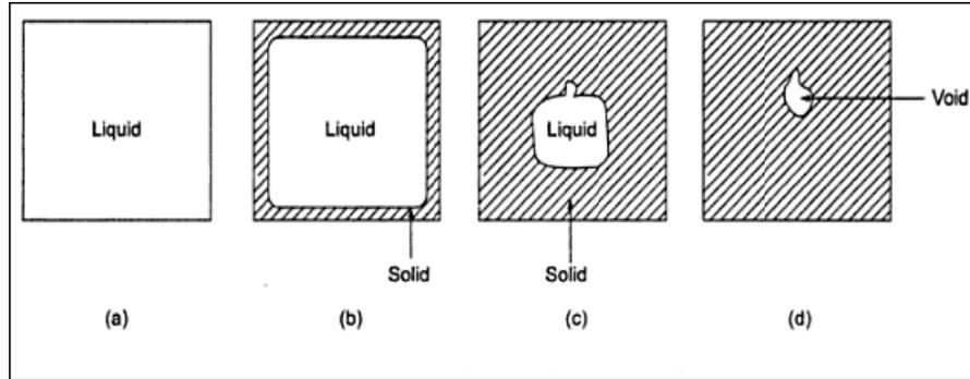
**Fig. 1. Formation of shrinkage cavity** <sup>[1]</sup>.
