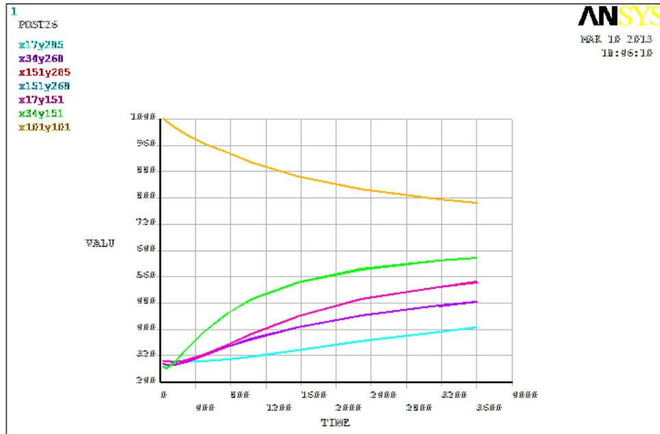
Fig. 12. Temperature Time Graph for PLANE 35 element
