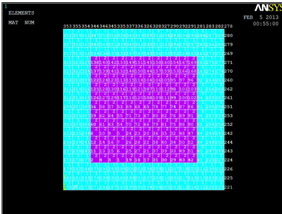
**Fig. 6 Mapped Mesh of Casting**
