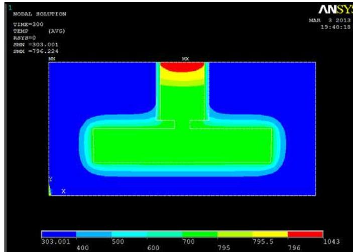
Fig. 17. Location of Hot Spot for Riser with Sleeve
