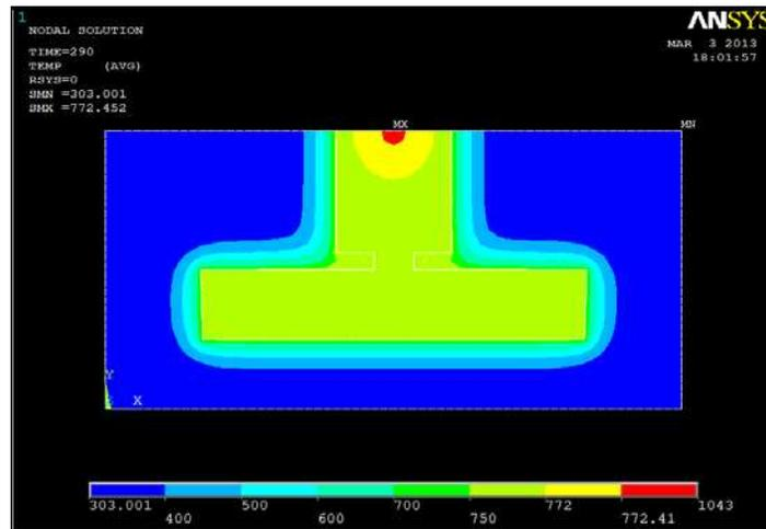
**Fig. 16. Location of Hot Spot for Riser with Diameter 60**
