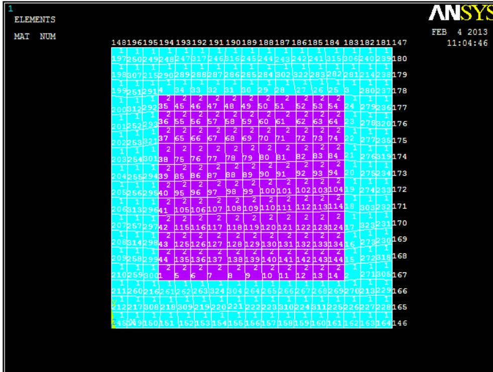
**Fig.5 Free Mesh of Casting**
