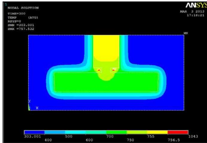
**Fig. 15. Location of Hot Spot for Riser with Diameter 50**
