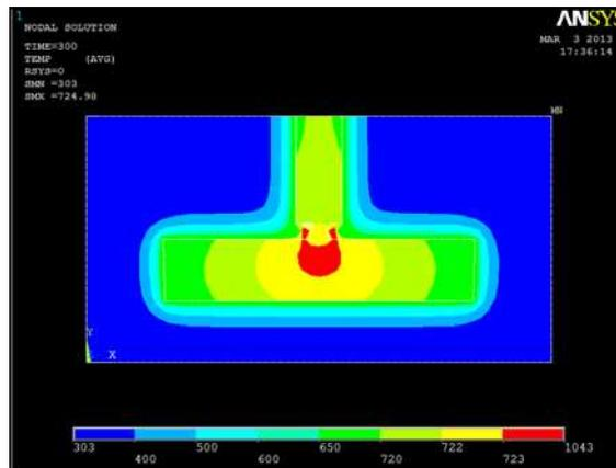
**Fig. 13. Location of Hot Spot for Riser with Diameter 30**
