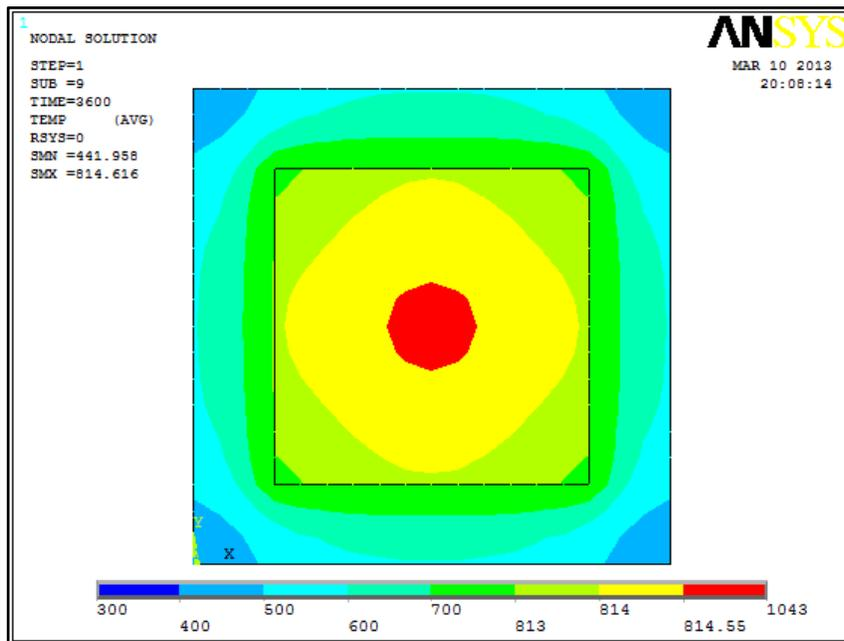
**Fig. 10. Location of Hot Spot in Mapped Mesh**
