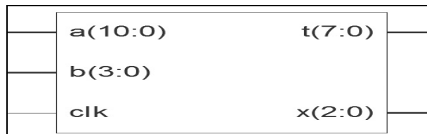
Fig 9: Black Box of CRC Checker
