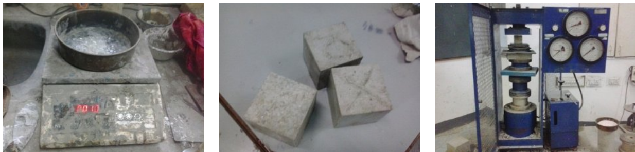
Fig.4 Casting of cubes, mortar cubes and testing of cubes
