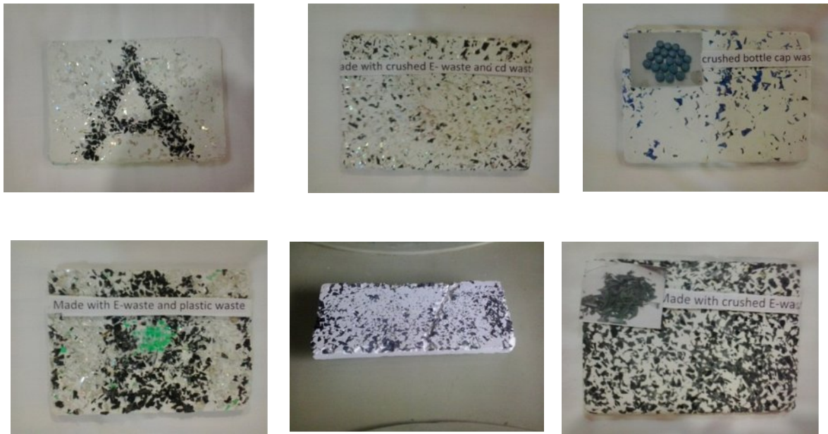
Figure 3: Tiles casted with white cement and waste material
