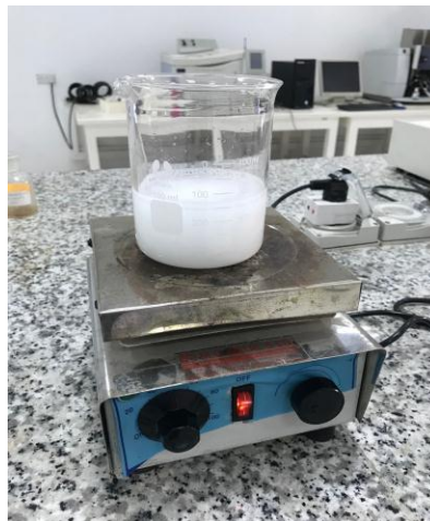
Figure 2 Nanofluid suspension on magnetic stirrer
