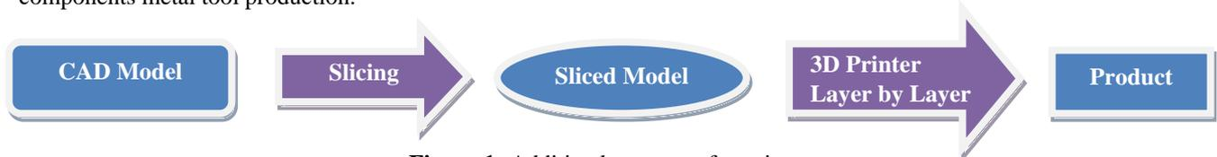
Figure 1: Additive layer manufacturing.
