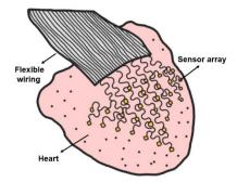
Figure 6: Schematic illustration of soft implantable device conformally attached to heart for ECG mapping.
