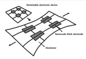
Figure 4: Schematic illustration of stretchable electronic device
