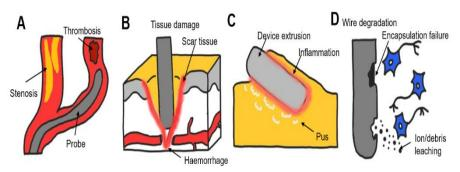
**Figure 2:** Schematic illustrations of side effects induced by conventional rigid bioelectronics including (A) stenosis and thrombosis, (B) tissue damage by wire implantation, (C) pus and pain due to subcutaneous implantation, and (D) wire degradation by body fluids.
