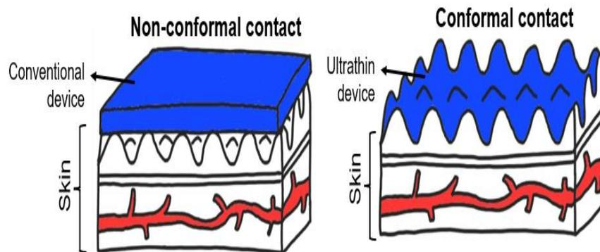
**Figure 3:** Schematic illustration of interface between electrode and skin.
