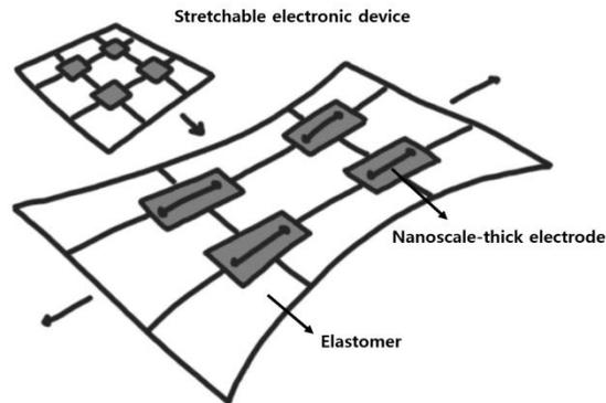
**Figure 4:** Schematic illustration of stretchable electronic device
