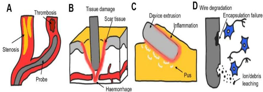
**Figure 2:** Schematic illustrations of side effects induced by conventional rigid bioelectronics including (A) stenosis and thrombosis, (B) tissue damage by wire implantation, (C) pus and pain due to subcutaneous implantation, and (D) wire degradation by body fluids.
